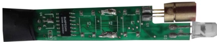
Figure 2.20: laser with k2 button bypassed
